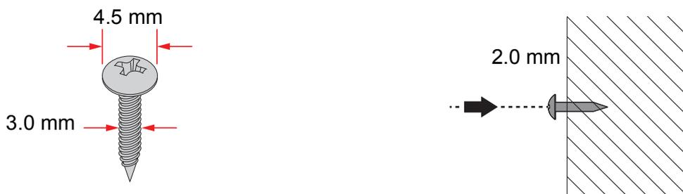
**Figure 2.4 Securing Wall Mounting Screws**
