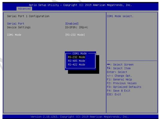
6. When the mode is set to RS-485, "auto flow control" will be automatically enabled. Users don't need to change it additionally.
