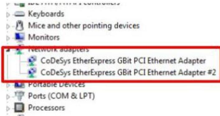
Path of driver: C:\Program Files\3S CODESYS\CODESYS Control RTE3\CmpEt1000MPD\
