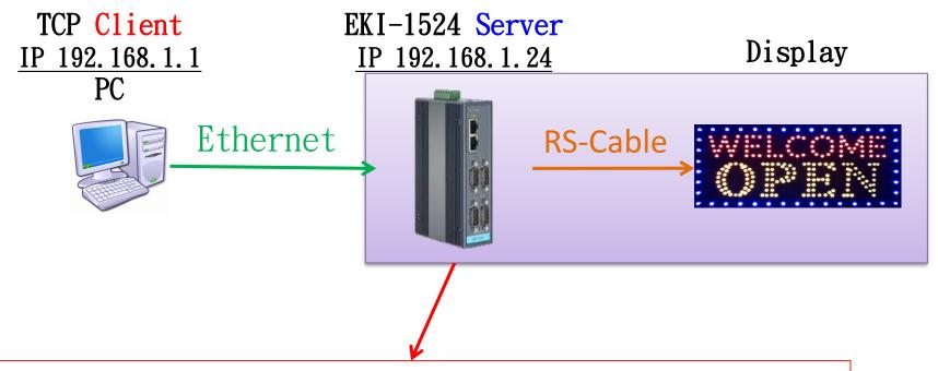
Device server is using the TCP port to listen the data from the client over the Ethernet.
