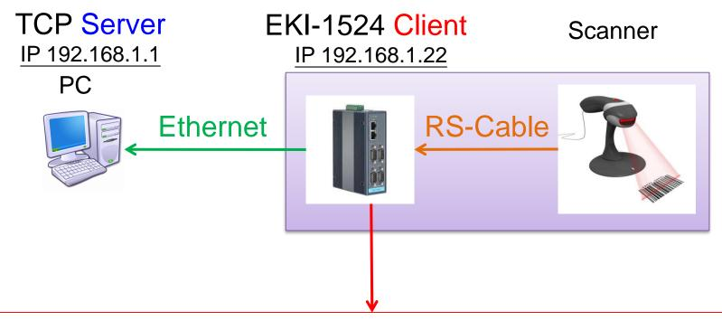
In the initial connection, Device server send data by RS-Cable After connected, data can be sent by both side
