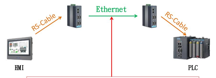
In this topology, the data is sent from left side to right side. So, TCP Client is the left device server, TCP Server at the right side.
