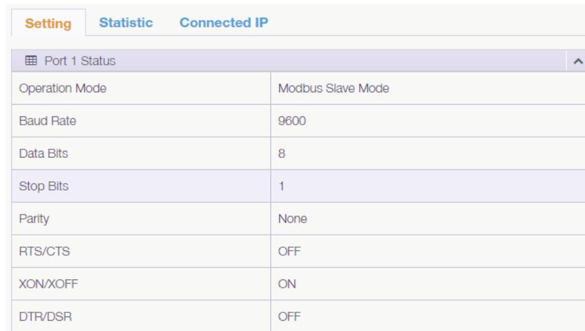
The screenshot shows a web interface with three tabs: 'Setting' (selected), 'Statistic', and 'Connected IP'. Below the tabs is a table titled 'Port 1 Status'. The table has two columns: 'Item' and 'Value'. The items and their values are: Operation Mode (Modbus Slave Mode), Baud Rate (9600), Data Bits (8), Stop Bits (1), Parity (None), RTS/CTS (OFF), XON/XOFF (ON), and DTR/DSR (OFF).
