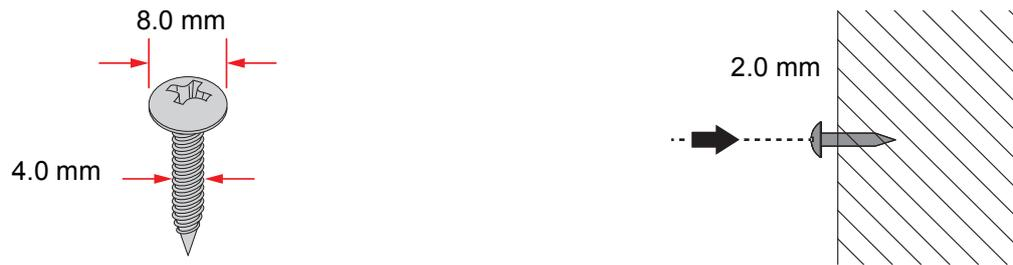
**Figure 2.34 Securing Wall Mounting Screws**
