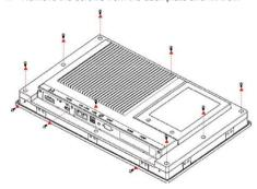
2. Remove the screws from the blanking plate.
