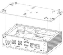
2. Insert the mini-PCI card and secure with the screws.
