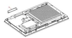
3. Insert the PCM Module through the open slot.
