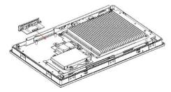
4. Secure the PCM Module with the screws you removed from the blanking plate.
