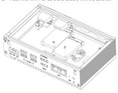
3. Remove the screws to remove the blanking plate.
