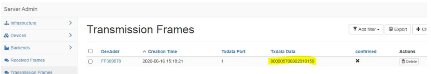
**Figure3:** The downlink command generated by application server
