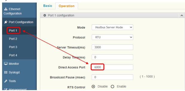
Set ModScan connection detail to TCP service port from port 6000~6003, according to the target COM port.
