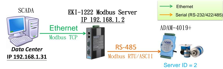
*SCADA (Data Center)* polls data through Modbus TCP. The EKI translates the data from TCP to RTU, and send to end device. Then end device responses data to *Data center*.
