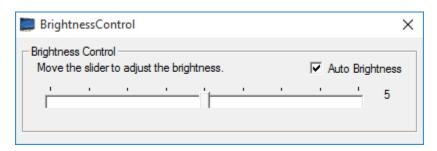
You can move the slider to adjust the brightness. If the target platform supports Auto-Brightness function, the UI will show the "**Auto Brightness**" check box as previous figure. If the Auto Brightness check box is checked, the brightness slider will be disabled.
