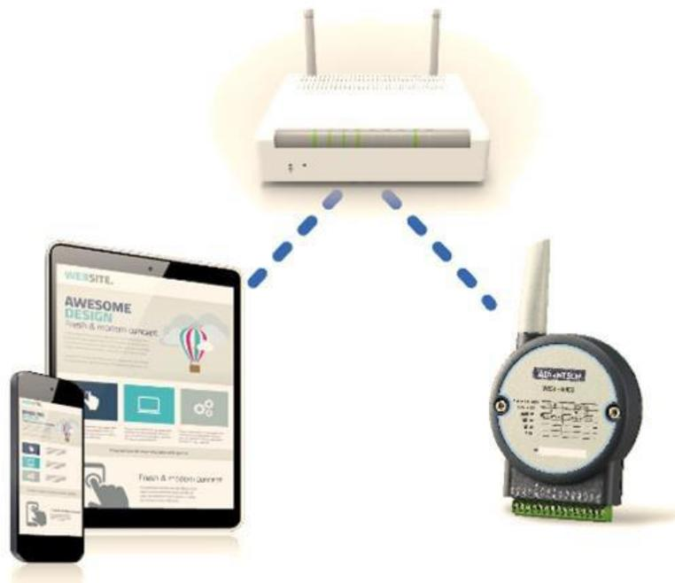
Unlike the limited AP mode which allows only one device connected to WISE at the same time, multiple different devices can connect to the AP and monitor the data of WISE at the same time.
