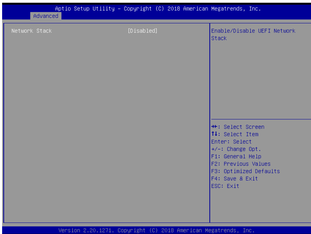
Figure 3.33 Network Stack Configuration
