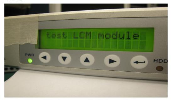
2.1 To open the terminal and type the command "./lcmap 378" and press enter.
