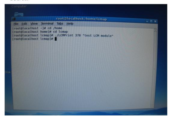
1.2Then the LCD will show the message that you type, "test LCM module"
