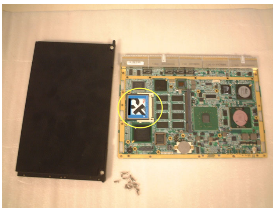
Figure 1.9 Insert the CF card in CN10
