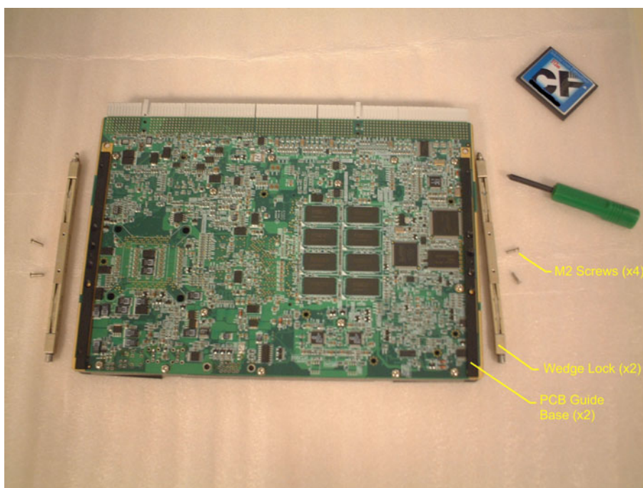
Figure 1.4 Remove the wedge locks from the conduction-cooled plate
