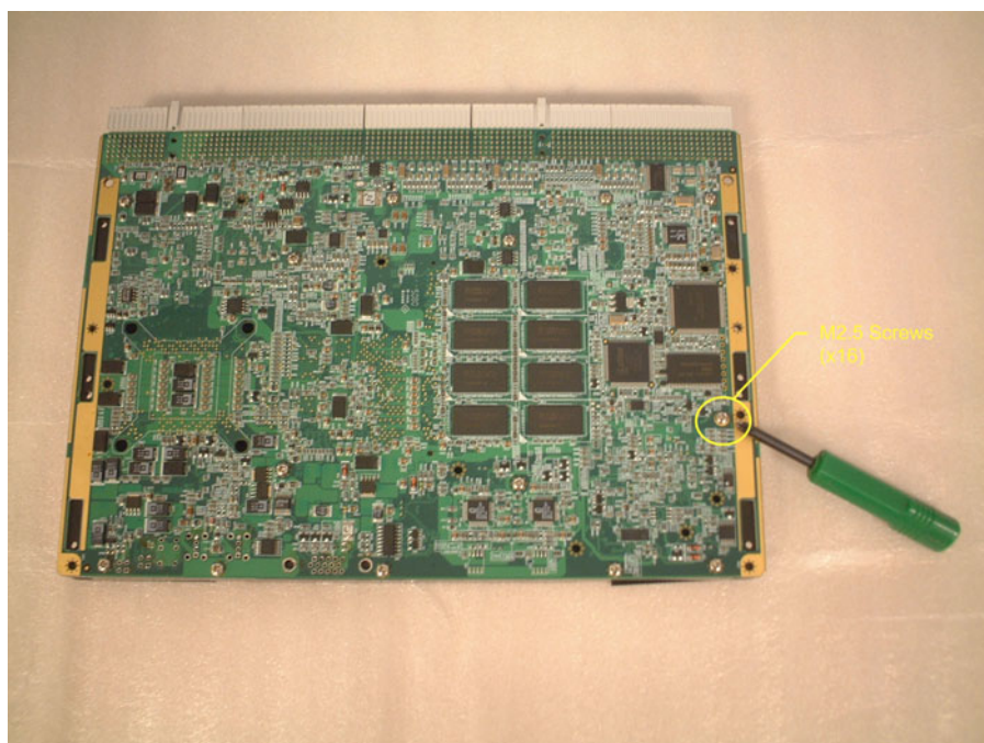
Figure 1.7 Remove the M2.5 screws from the secondary side of the PCB
