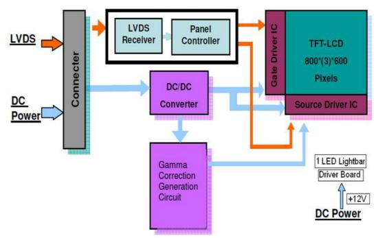
Figure 1.1 Function block diagram
