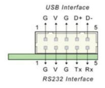
Figure 5.1 Board mounted header
