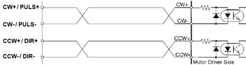
Figure 3.4 Photocoupler Interface
