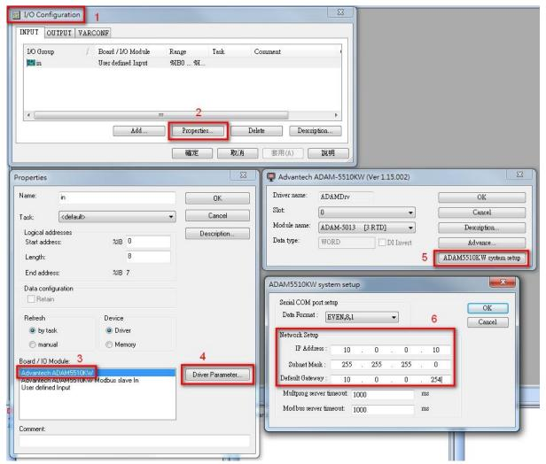
**Step 4**: Rebuild the project then download the project with IP changed setting to ADAM-5510KWTP and cold restart. Furthermore, you need to click reset button to reboot the ADAM-5510KWTP. After system reboot, the new IP address will be effective. Then you can change new IP address in resource setting to connect the ADAM-5510KWTP.
