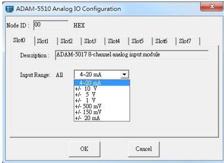
**Step 5:** Configure each IO then remove the “initial pin” then reboot ADAM-5510 series.
