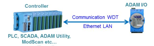
When the communication is down, with the help of communication WDT, user can turn on or turn off the output within a particular period to prevent unstable or dangerous output status.
