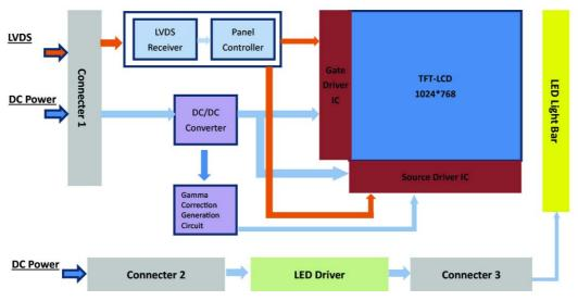
Figure 1.1 TFT LCD module
